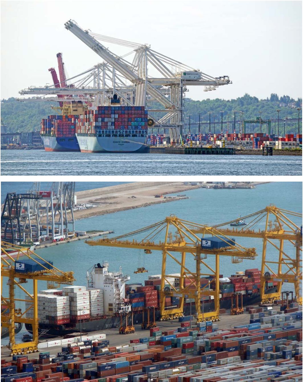
Figure 4.7. Dock workers called stevedores, or longshoremen, unload cargo containers from freight vessels using giant gantry cranes that grasp the containers with a “spreader.” The spreader lifts the containers over the ship rail and shuttles them to the dock. Ports of Seattle, Washington (above) and Barcelona, Spain (below).
