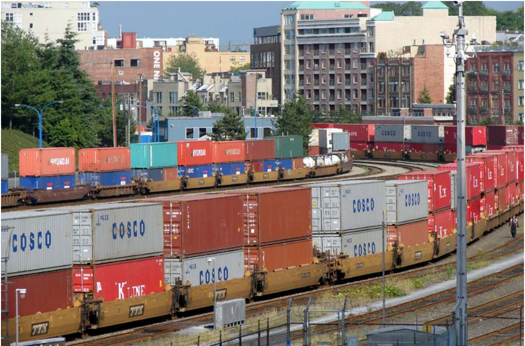
Figure 4.12. Train yards like this one in Vancouver, Canada, frequently run directly through a major port. Cranes or lifts load the isotainers from the dock onto special train cars designed to hold the isotainers. To save space, isotainers may be stacked two high, as here.
