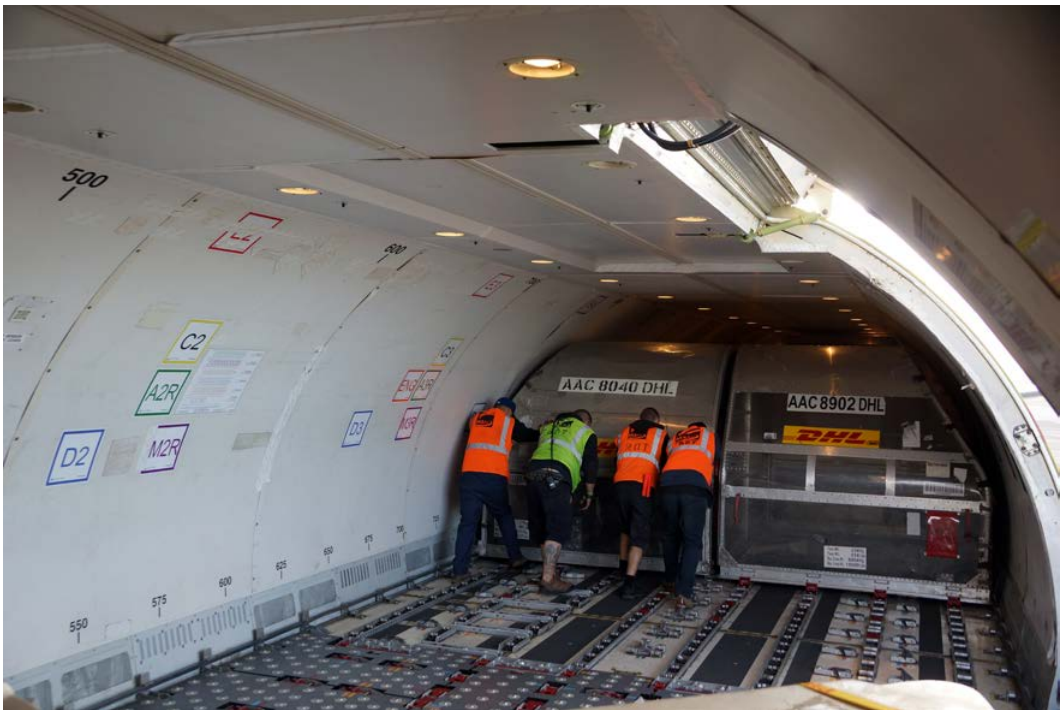
Figure 4.10. Air freight being loaded into a commercial freight airplane's cargo bay. © 2013 by Aaron X. Fellmeth
