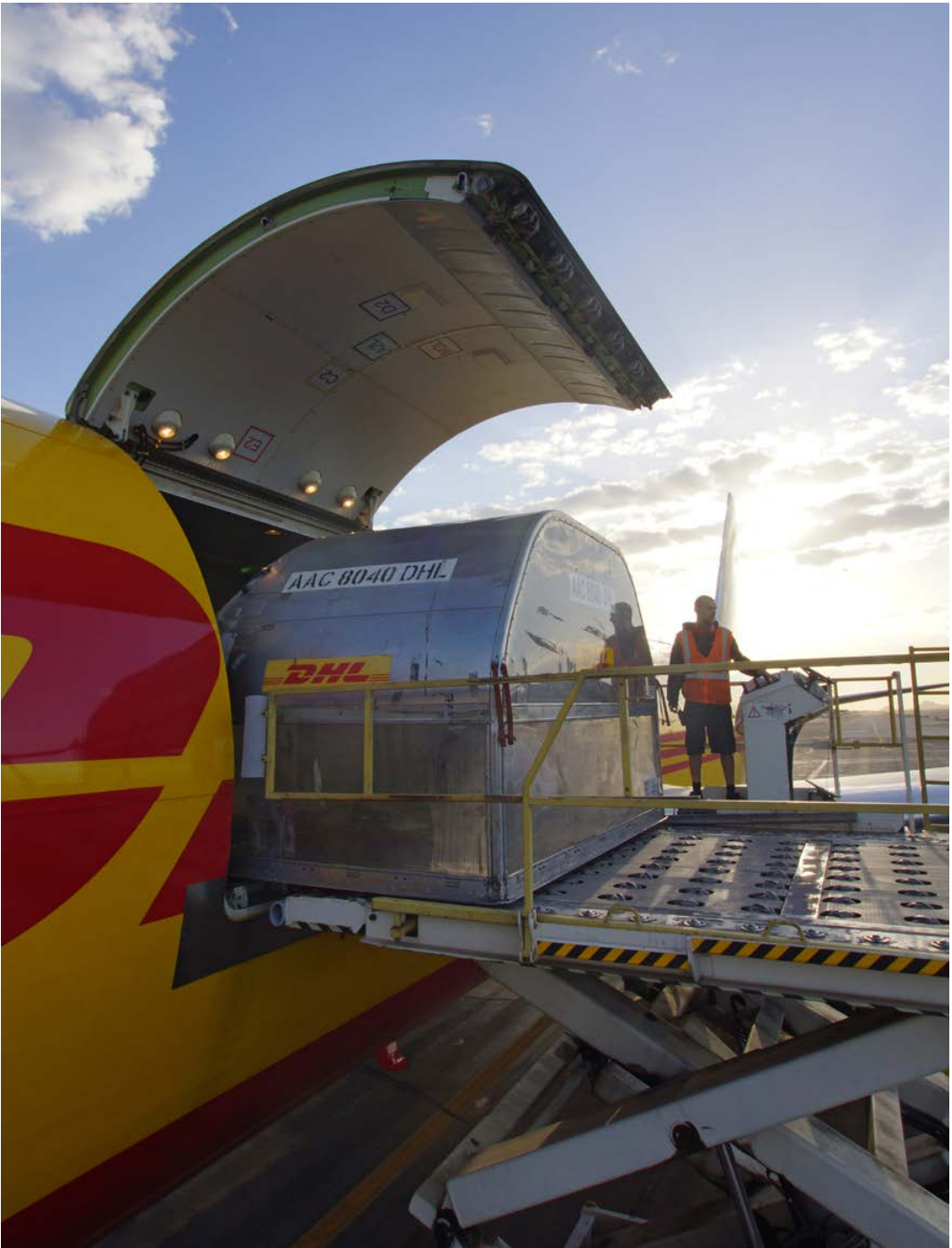
Figure 4.1. A cargo airplane loads freight into the top half of the hold using an electric lift. The hold in a cargo plane comprises most of the fuselage and is divided into upper and lower halves. Notice how the cargo container is rounded on top to fit in the top half of the airplane's cylindrical fuselage. © 2019 by Aaron X. Fellmeth
