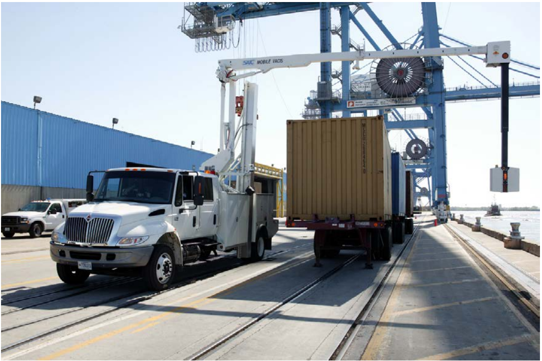
Figure 5.7. Customs and Border Protection uses an advanced X-ray to scan isotainers. Credit: James Tourtellotte, U.S. Customs & Border Protection
