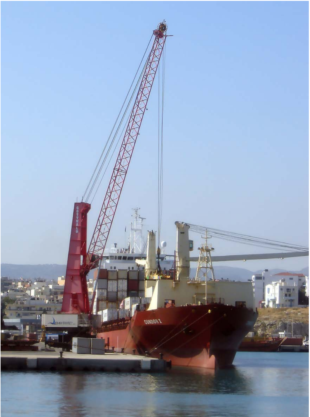
Figure 4.8. On the waterfront. In smaller ports, like Irakleio, Crete (Greece), derrick jib cranes rather than large gantry cranes are used to load and unload cargo.
