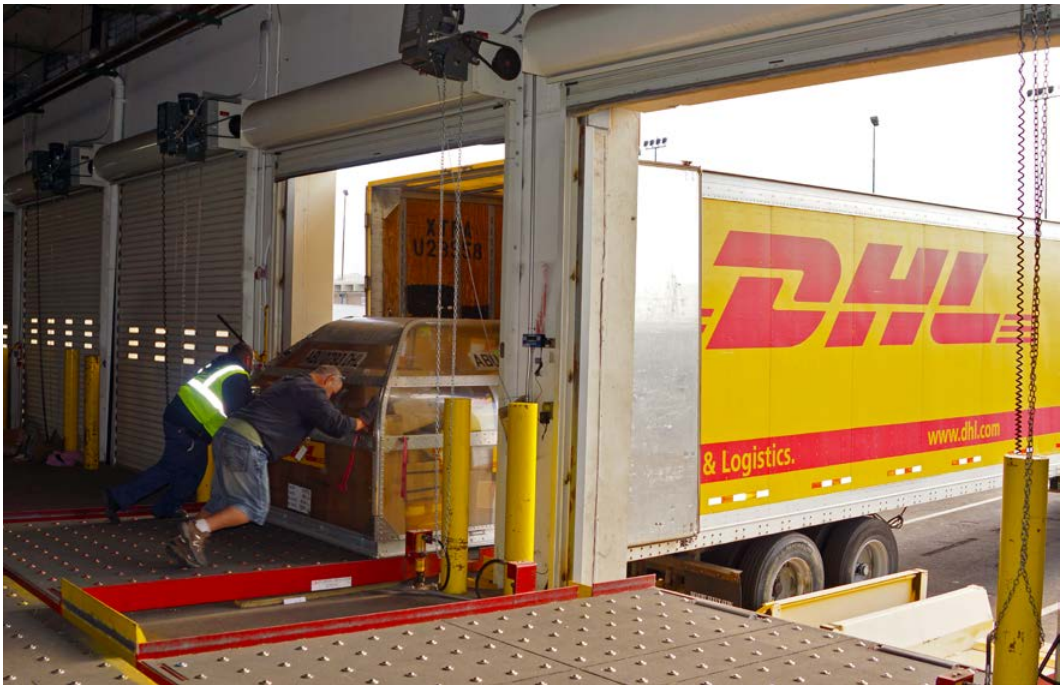
Figure 4.13. An air cargo isotainer being loaded onto a truck for ground delivery out of Sky Harbor Airport, Phoenix, Arizona.
