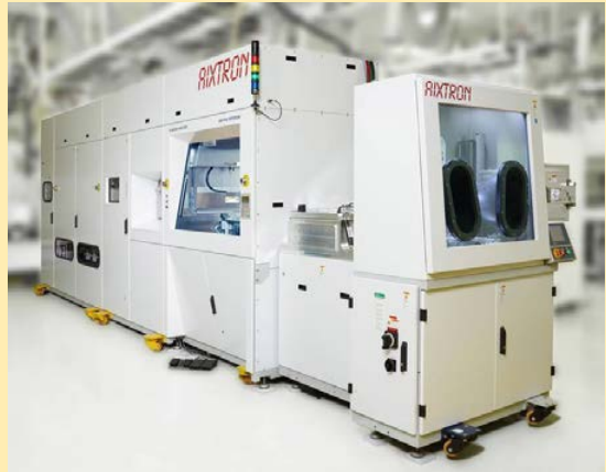
Figure 7.4. An Aixtron machine for depositing thin films on semiconductor wafers. Credit: © 2015 by Aixtron SE
